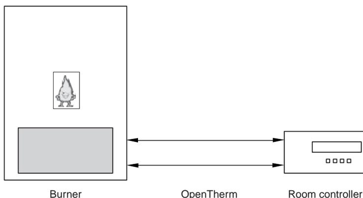
There are two different protocols for OpenTherm, an analog one, which is called OT/- and the digital one called OT/+. Some devices supports both and have to detect automatically the protocol used by the partner-device. This is done after reset/restart of the room-controller by communication time-out regarding the OT+ protocol.
